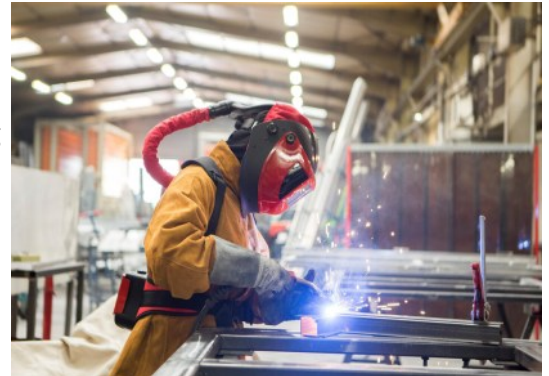
An example of personal fume protection
