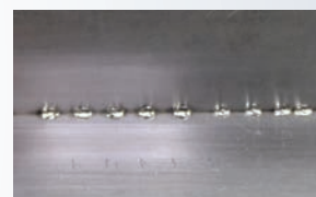
Corner spot welding thickness 0,6 mm
