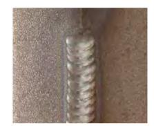
WELDING POSITION: HAC gives an optimal fusion of the bead's edges in short arc welding and to make overhead and vertical up position welding easier.
