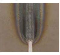
PG POSITION: HAC allows thin plates welding in vertical down position with gap up to 5mm wide.
