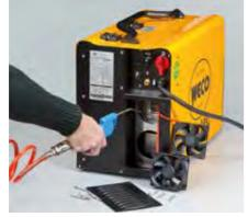
Ventilation grids and ventilators removable to allow an easy cleaning of the heat sink, by means of compressed air.
