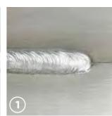
LEVEL 3: A low current ends LEVEL 2: The welding LEVEL 1: A correct initial gives filling the crater on weld the plate thickness and the penetration from welding start.
