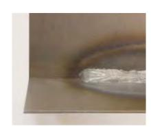
THIN PLATES: HAC gives smooth and controlled short arc at lower parameters too. Low spattering, good edge wetting, low heating and small deformation are achieved in thin plate welding.
