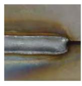
**SOFT START:** Approaching speed of wire and welding dynamics are totally synergic giving low spattering at start, in any type of material.
