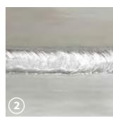
the welding optimally by current is optimized with current requested weld.
