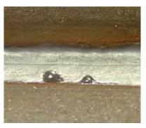
SPRAY ARC: HAC allows you to have a short spray arc with better penetration of the root, lower heat input and higher welding speed with no edge cutting and spattering.
