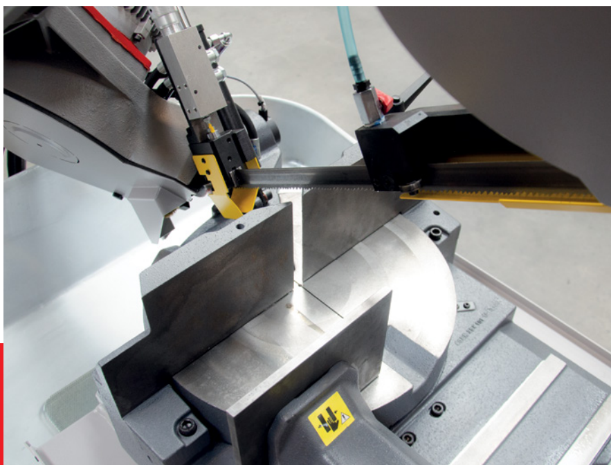
Sturdy rotary table enabling material to be cut at an angle without debasing the finishing plate.
