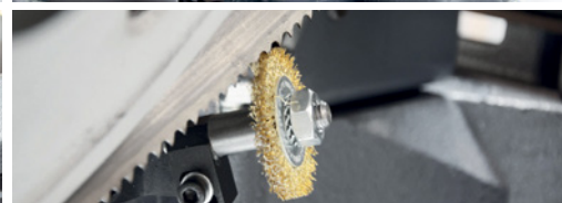
A chip brush is always driven concurrently with the speed of saw blade in order to provide an ideal cleaning effect.
